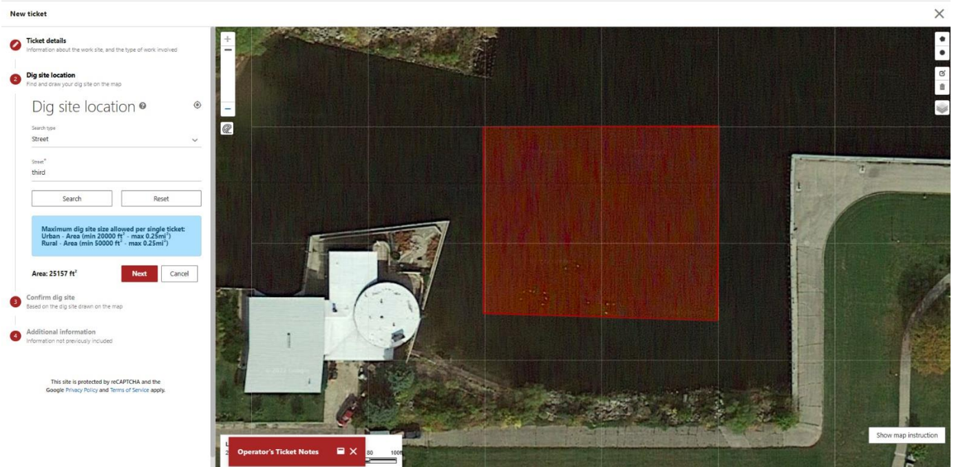
(Figure 2: With OneCallAccess the excavator can now solely place the polygon in a body of water as the excavation site. GPS coordinates can also be used to easily identify the excavation location. GPS will be a useful tool when excavation occurs in a large body of water where no other identification marks around.)
